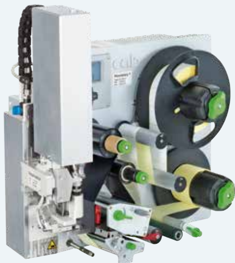
Hermes+ with stroke applicator 4114
